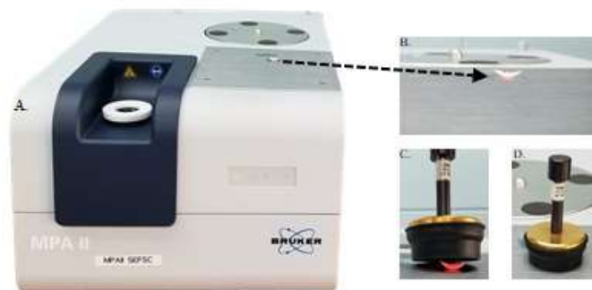
Near-infrared spectrometer (A). Otolith ready for analysis (B). A gold-coated reflector stamp covers the sample during scanning (C, D). Photo: NOAA Fisheries.
